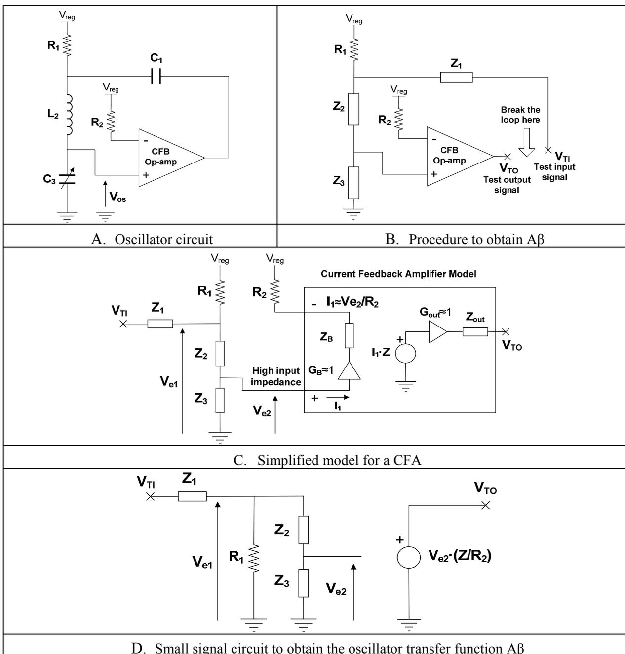
$$\frac{V_{TO}}{V_{TI}} = \frac{Z_3 \left[ \frac{R_1 \cdot Z}{R_2} \right]}{(R_1 + Z_2 + Z_3) Z_1 + (Z_2 + Z_3) R_1} \quad G = \frac{R_1 \cdot Z}{R_2} \quad (5)$$
