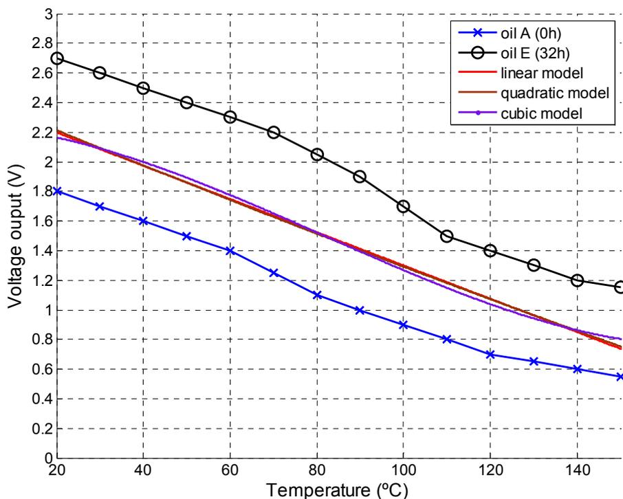
The same procedure for temperature compensation can be applied to a specific machine lubricant. The experimental dataset consists on lubricant samples at different degradation stages and sampling time intervals. As a result, a custom based calibration approach could be performed providing a more meaningful indication of the oil condition for a specific industry asset.
