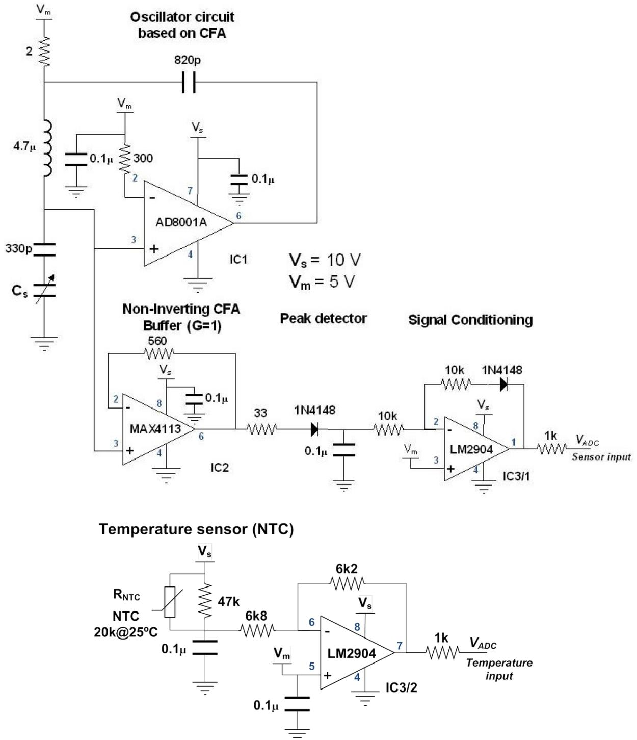
2.2.1. Oil Temperature Sensing Circuit
