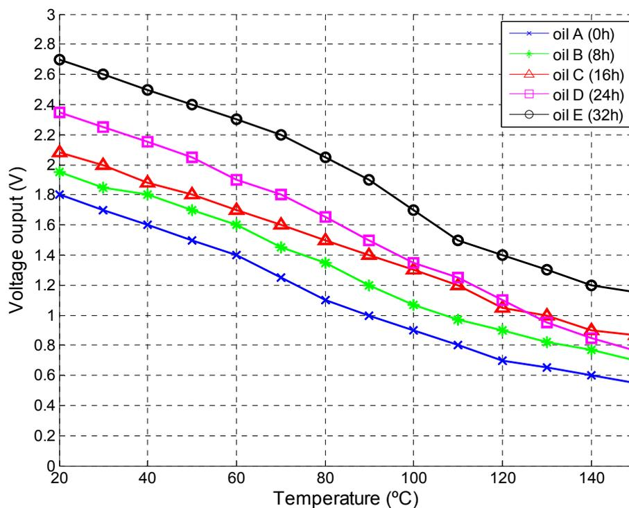
At a given temperature the output voltage is proportional to the oxidation stage. The experimental data in Figure 12 is curve fitted to different regression models in order to obtain the temperature dependency of the sensor's output. As shown in Figure 13, a linear model fits the data (5 datasets) with a good degree of accuracy ( $m = -0.01123$ ,  $b = 2.422$ ). The selected model can be implemented in a MCU to compensate temperature drifts due to temperature variations.
